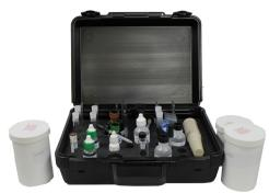
**438 Test Kit** Tests for Hardness, pH, Iron, Manganese, Tannin, H2S and TDS
