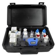
**2059 Test Kit** Tests for Hardness, pH, Iron, Tannin, H2S, Chlorine and Nitrate
